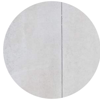
INSITU CONCRETE PAVING 03 (OPEN SPACES) 150 U5E insitu concrete 10mm basalt oxide
