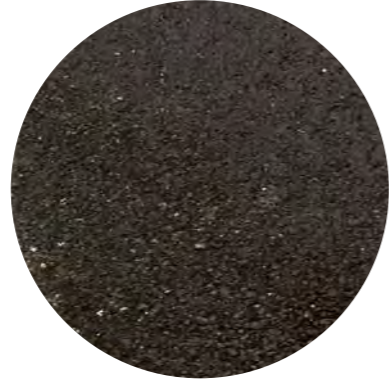
ASPHALT PAVING City Mix10 (TNZ-M/10 spec) for cycleway areas
