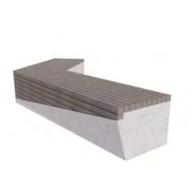
PRECAST CONCRETE SEAT Precast concrete seat purpleheart timber battens, gauged and chamfered to cover top and side of concrete plinth with skate deterrents
