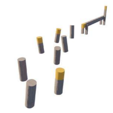
PLAY TRAIL Beam and stepper logs (use site won timber where available)
